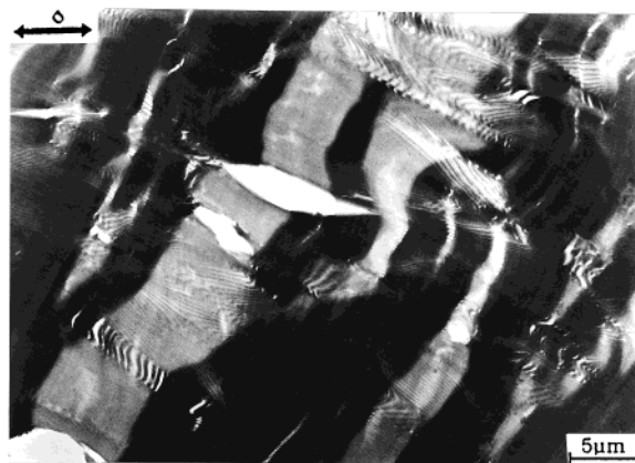
Figure 6. HVEM micrograph of deformation zones of an intermediately segregated PS- b -PBMA diblock copolymer at \chi N = 39 already discussed in detail in our previous study 23 ( \Phi_{\text{PS}} = 0.70 , M_n = 315 \text{ kg/mol} , lamellae). The craze propagation is influenced by morphology and does not occur perpendicular to the external stress direction in all cases.
